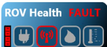
Sample ROV Health Indicator displaying a communications fault.
