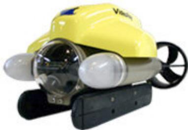
The Pro 4 Ultra ROV (Remotely Operated Vehicle) is depth rated to 300 meters (1000 feet).
