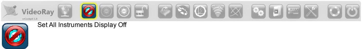
There are three buttons on the control bar to manage the display properties of instruments. You can turn off all instruments, make them all transparent, or make them all opaque. These buttons work on all instruments as a group rather than individually.
