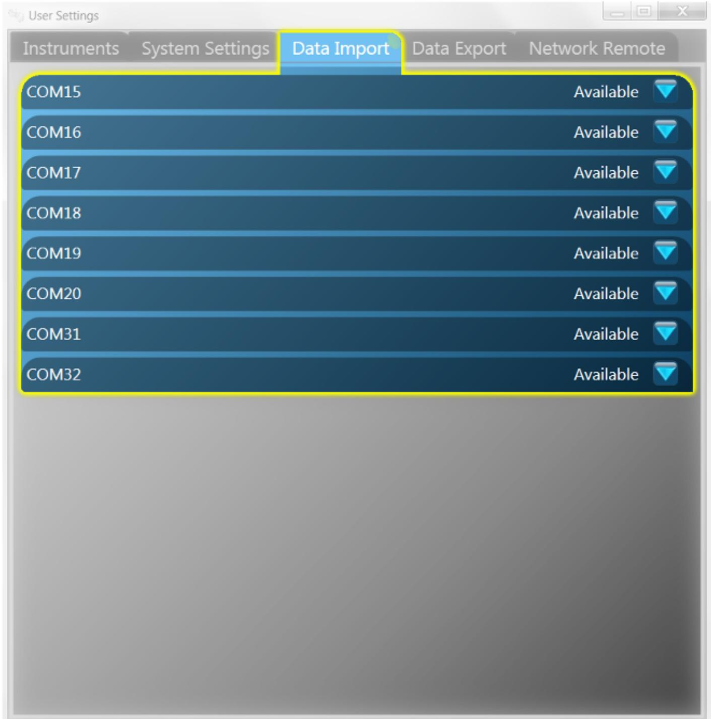
Data Import reads data from a COM port. Either a physical COM port or virtual COM port can be used. Virtual COM ports can be used to allow two programs on the same machine to talk to each other. An example might be to have the KCF Smart Tether send the ROV position data to VideoRay Cockpit, so that the position of the ROV can be recorded as overlay text on the video image. See the [Application Integration](#) section for more information about virtual COM ports.
