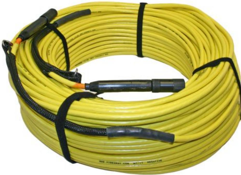
Tether connects the ROV to the surface and provides power, communications, video and an APIC (Auxiliary Pair of Independent Conductors) for accessory use. The tether consists of conductors, a Kevlar® strength member, flotation (for Neutral and Performance tethers) and an outer jacket. It is available in three types: Negative, Neutral and Performance (often called PPT). Neutral and Performance are neutrally buoyant in fresh water because they have a specially designed foam jacket.
